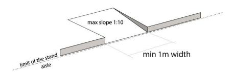
Level landings must be provided at the top and the bottom of the ramp and at every intermediate level where an exit door can be opened.
