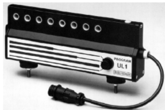
Fig. 108 – Piezoelectric electronic weft stop motion with integrated amplifier, which at its output emits two logic signals to indicate the broken weft or weft excess in the insertion.
