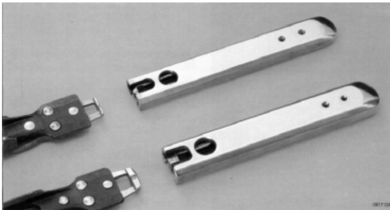
Fig. 45 – Projectiles : there are various projectile versions: made of steel, 9 cm long and 40 g heavy, with small section, as suitable for yarns of fine to medium count; made of steel, 9 cm long and 60 g heavy, with large cross-section which, thanks to their higher weight and to the larger clamping section of the gripper, are particularly suited for machines with high reed width or when for weft bulky yarns, as e.g. fancy yarns, are used.
