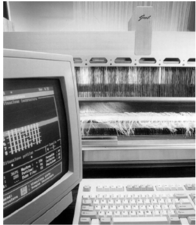
Fig. 31 – A harness and a reed with drawn-in threads ready to be moved to the knotting station.
