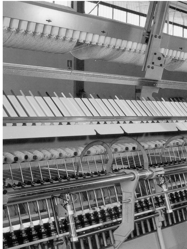
Fig. 100 Tubes orderly positioned on the rack
