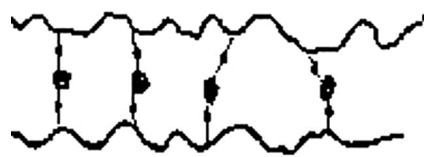
Fig. 184 Polyglucose chains cross-linked with thermosetting resins
