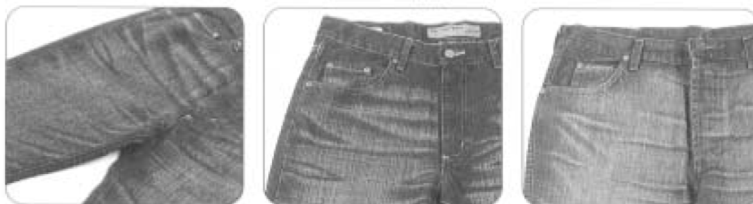
Effetto graffiato tramite raggio laser + Scrapping effect by laser treatment
