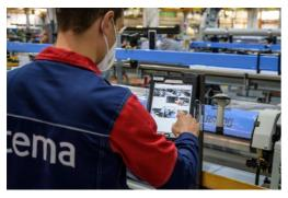
A phase of the manufacturing of the Itema weaving machines in the Colzate plant. The operators, through tablets and scanners, have all the data of the machine assembly according to the principles of industry 4.0
