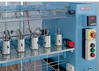
The 1700/20 machine is suitable for the production of any kind of tripolino, whether for passementerie, knitwear production, accessories and in many other sectors including the medical field. This machine is especially designed for the production of elastic, resistant and soft to the touch chainette cords. The specifications of these elastic cords enable easy connection to the fabric and make them ideal as ear loops for protective face masks, both disposable and reusable.
