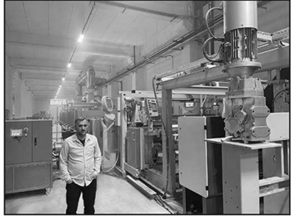
The coater is installed at the front of the eighth Monfongs Montex stenter supplied to the company.
