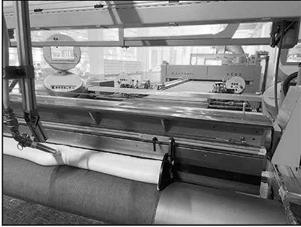
The Montex®Coat unit enables an even foam application to be achieved at high speeds.
