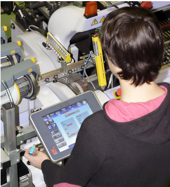
Fig 2: the touch screen console allows the weaver and the technician to operate the Silver 501 in a very user friendly way.
